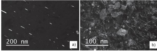
**Figure 3.** A typical dislocation structure with radiation defects in a RVI steel sample after irradiation: **a)** dark-field images of Frank's dislocation loops; **b)** blackdots-type defects.
