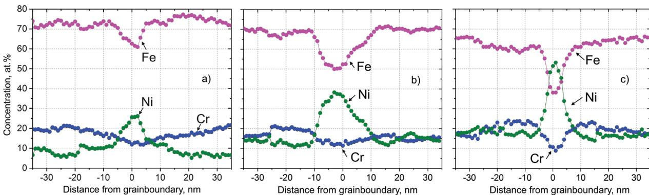
**Figure 6.** Typical chemical elements distributions near the grain boundaries, obtained by the STEM method in the EELS mode in RVI steels with various Ni contents: 10 (a), 20 (b) and 25 wt.% (c).
