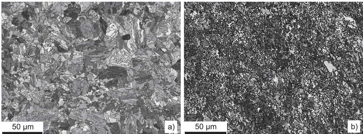
**Figure 1.** Orientation distribution (EBSD) maps of the substructural elements separated by high-angle boundaries in the RPV steels with Ni contents of 1.5 wt.% (a) and 5.2 wt.% (b).
