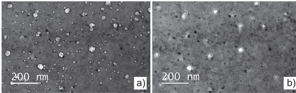
**Figure 5.** Typical TEM image of voids under underfocusing (a) and overfocusing (b) condition in a RVI steel sample after irradiation in the BOR-60 reactor at 425 °C to a irradiation dose of 29 dpa.
