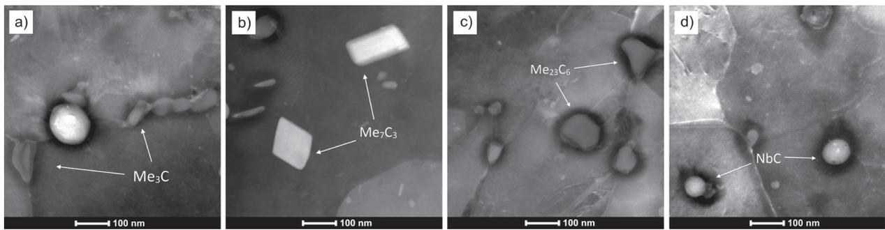
**Figure 2.** Typical STEM images of large carbide precipitates found in the examined RPV steels.
