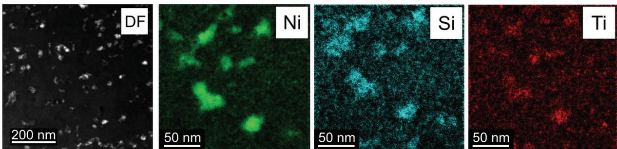
**Figure 4.** Typical dark-field TEM (DF) image of a G-phase and corresponding element distribution maps (Ni, Si, and Ti) obtained by energy-filtered TEM.
