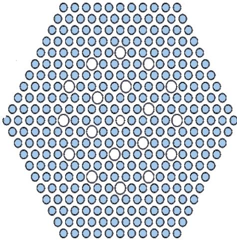
**Figure 1.** Horizontal cross section of the fuel assembly of the VVER-1000 reactor.
