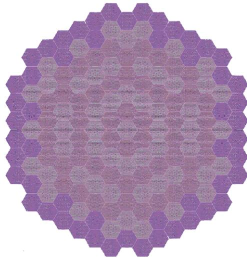
**Figure 2.** Core consisting of three sections with different burnups. Purple color indicates “fresh” fuel assemblies (Section 1), gray color indicates fuel assemblies after one year of reactor operation (Section 2), pink color indicates fuel assemblies after two years of reactor operation (Section 3).
