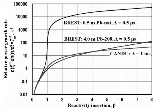
**Figure 2.** Relative rate of increase of reactor power depending on the introduced reactivity for lead-cooled fast reactors equipped with different reflectors and for CANDU-type reactor.
