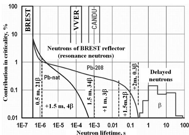
**Figure 1.** Contribution of neutrons with different lifetimes in the criticality of fast and thermal reactors.
