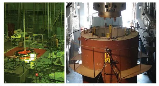
Figure 2. SM-3 reactor core withdrawal. a. From the reactor cavity; b. Loading into the K-1 cask.
