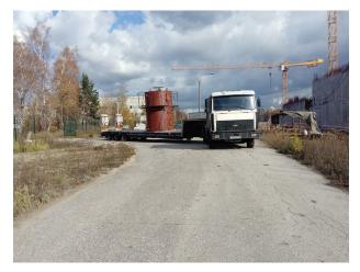
Figure 3. Transportation of the K-1 cask with the loaded reactor core.
