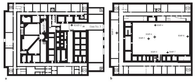
Figure 6. Positions of the radiation monitoring points inside the reactor building: a. Elevation +0.0 m; b. Elevations +8.4 m and 13.2 m.
