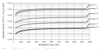
**Figure 5.** Induced activity of <sup>60</sup>Co in the reactor core structural components as a function of irradiation time: 1 -lower end parts of beryllium blocks; 2 -upper support plate; 3 -vessel between elevations of -200 and 200 from the core mid position; 4 -vessel outside elevations of -200 and 200 from the core mid position; 5 -lower end parts of beryllium blocks; 6 -bottom shell.
