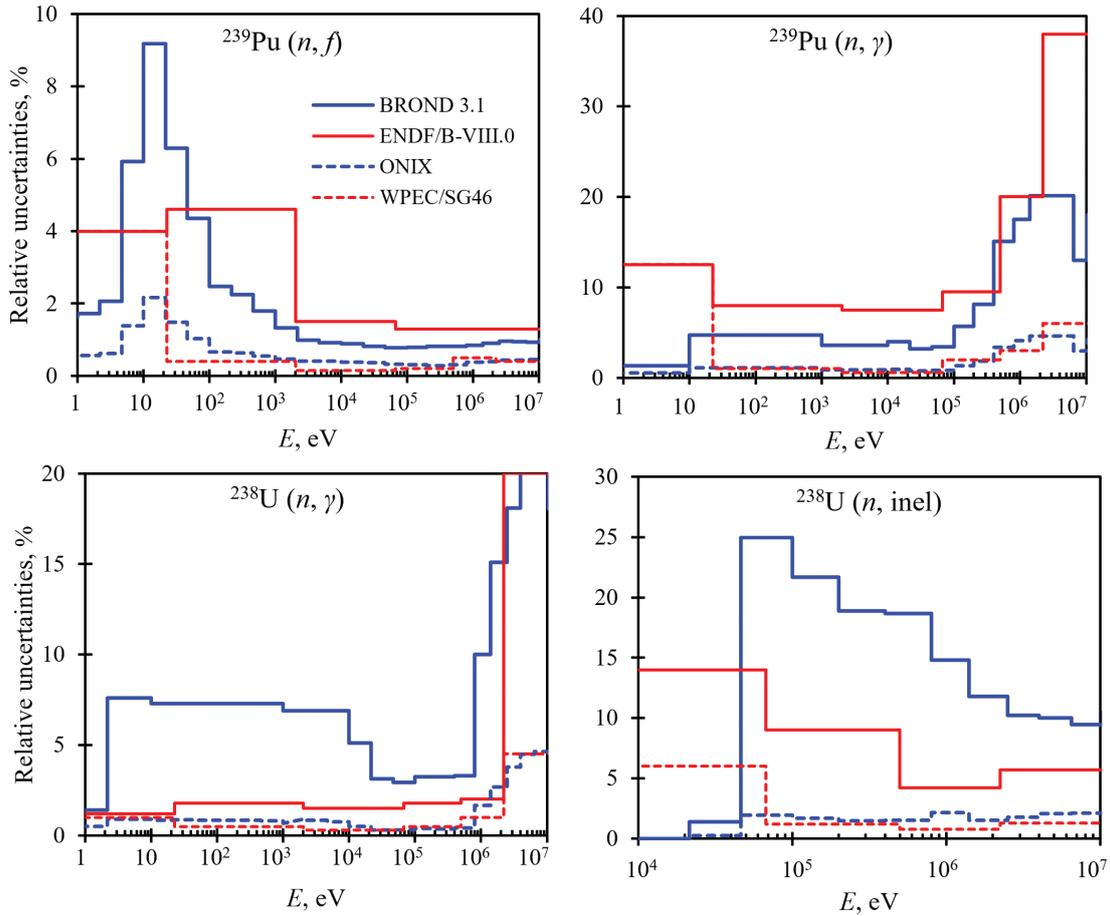
**Figure 1.** Relative uncertainties of important neutron reactions defining the  $k_{\text{eff}}$  uncertainty for a lead-cooled fast-reactor model due to nuclear data uncertainties (solid lines – uncertainties achieved, dashed and dotted lines – uncertainties required).
