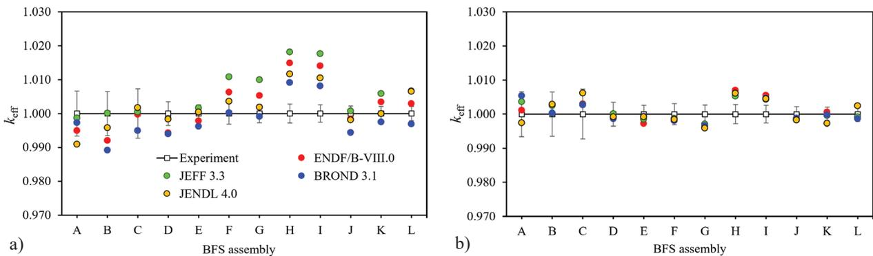
**Figure 2.** Calculation and experimental discrepancies in  $k_{\text{eff}}$ : prior to (a) and after (b) the neutron data adjustment. Letter designations for BFS assemblies: A – BFS-35-1; B – BFS-38-2; C – BFS-42; D – BFS-97-1; E – BFS-97-2; F – BFS-97-3; G – BFS-97-4; H – BFS-99-1; I – BFS-99-2; J – BFS-101-1; K – BFS-101-1; L – BFS-101-3.
