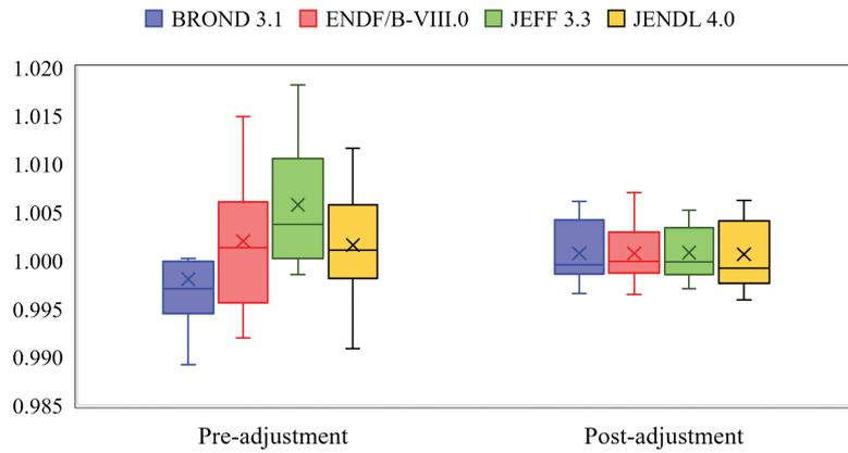
**Figure 3.** A priori and a posteriori  $k_{\text{eff}}$  uncertainties for the target system (for the case with a 30% content of plutonium in MOX fuel and a plutonium vector of 96, 4, 0, 0% for  $^{239,240,241,242}\text{Pu}$  respectively): crosses – mean value, line inside rectangular boxes – median, rectangular box boundaries – 25 and 75% percentile, whiskers – minimum and maximum values.
