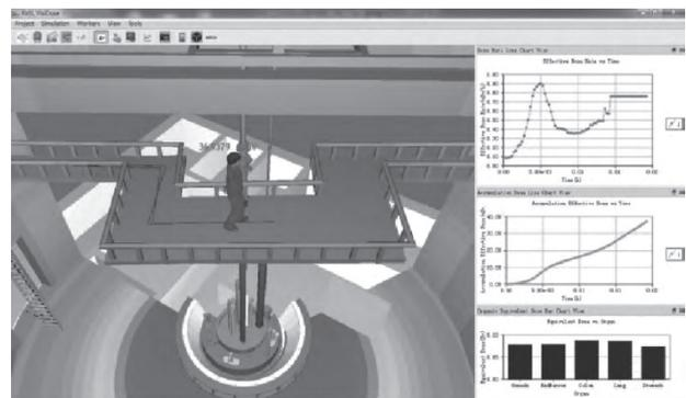
**Figure 9.** Display of the radiation field distribution in retirement scenarios for reactor decommissioning simulation system developed by NPIC.
