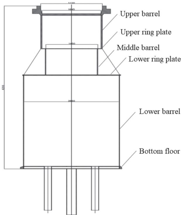
**Figure 16.** The structure of the outer shell of HWRR reactor.
