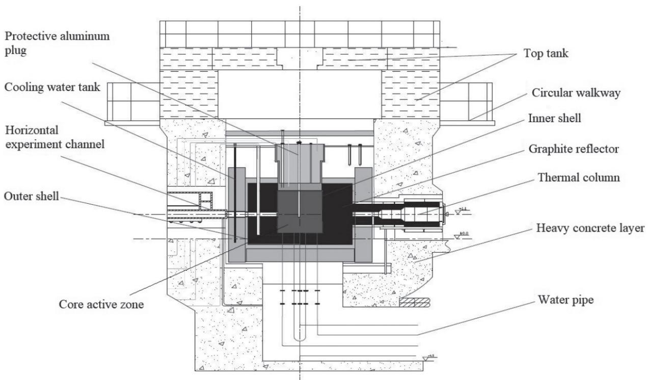
**Figure 15.** The main structure of the HWRR reactor.
