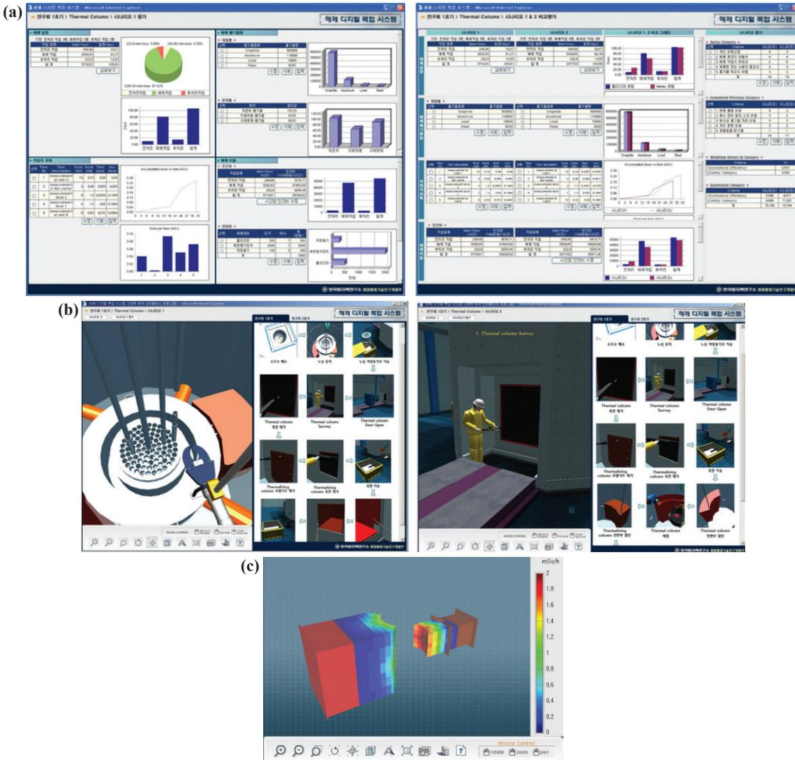
Figure 7. (a) Data management and calculation module of DMU code system; (b) Visualization display of model loading and simulation operations in DMU; (c) Visualization display of dose field distribution in a certain thermal column in DMU.
