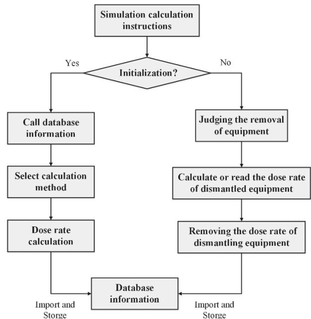
Figure 13. The calculation process of the dose field calculation program for HWRR reactor.
