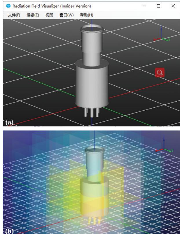
**Figure 17.** (a) Outer shell model of HWRR reactor; (b) Visualization display of dose field of HWRR reactor.
