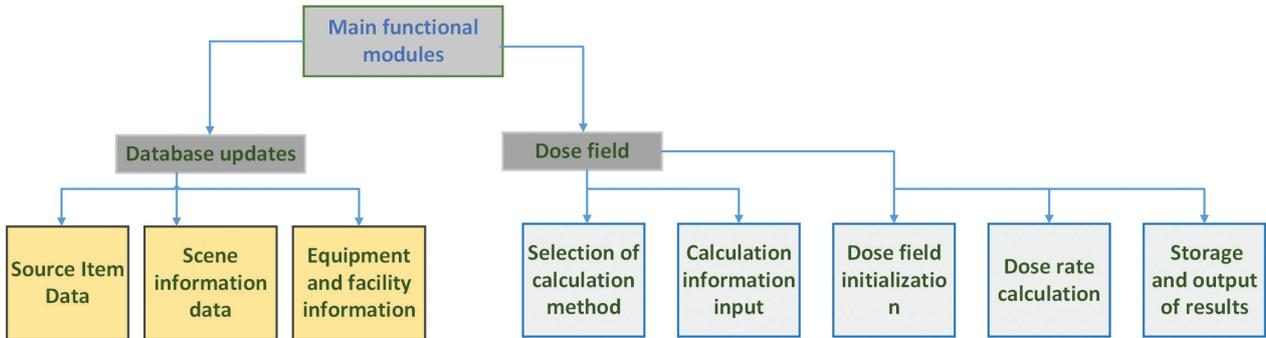
Figure 12. The main functions and module structures of the decommissioning dose field calculation code system for HWRR reactor.
