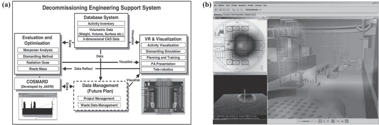
Figure 6. (a) System functional modules in DEXUS code; (b) Visualization display of a certain scene in DEXUS code.
