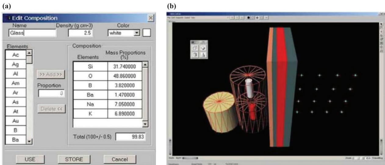
Figure 1. (a) Selection of multilayer shielding materials in MERCURAD code; (b) Visualization display in MERCURAD code.
