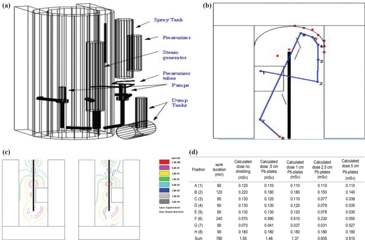
**Figure 5.** (a) Building the reactor model in VISIPLAN 3D-ALARA code; (b) Setting of personnel work trajectory in VISIPLAN 3D-ALARA code; (c) Dose field distribution when selecting different shielding materials in VISIPLAN 3D-ALARA code; (d) Calculation of the personnel exposure dose under different shielding materials in VISIPLAN 3D-ALARA code.
