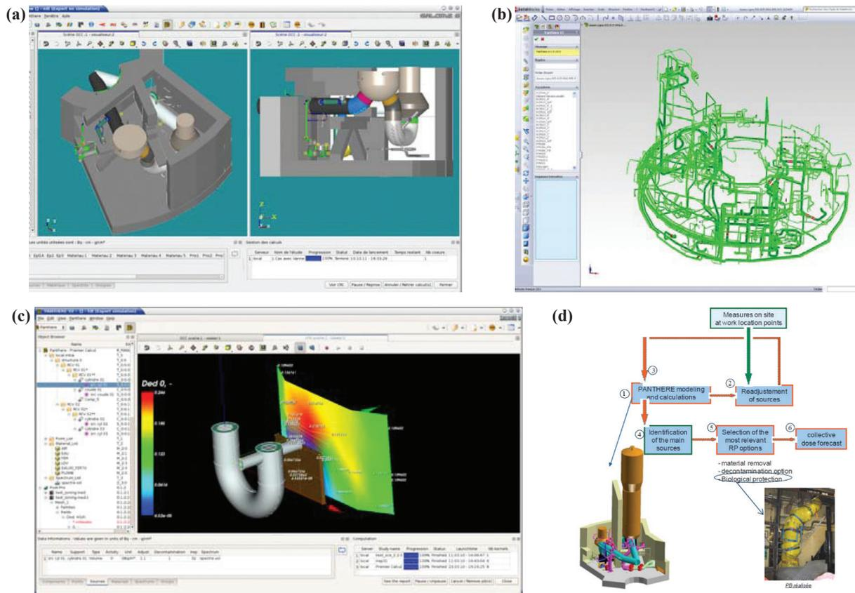
**Figure 4.** (a) Visualization model of a nuclear power plant in PANTHERE code; (b) Pipeline layout model for a nuclear power plant in PANTHERE code; (c) Visualization display of dose field in PANTHERE code; (d) Radiation optimization process in PANTHERE code.
