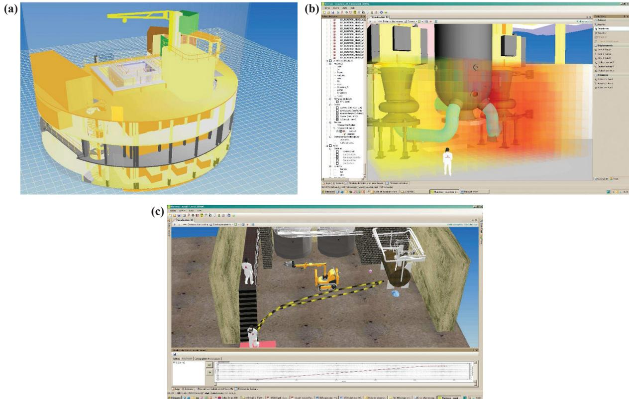
**Figure 3.** (a) Visualization display of a certain reactor model in NARVEOS code; (b) Visualization of the dose field in the personnel operating environment in NARVEOS code; (c) Dose rate display in personnel operation path in NARVEOS code.
